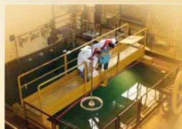
**POSEIDON** is a pool type industrial irradiator, able to store 37,000 TBq of Cobalt 60. The power of this irradiator is sufficient to obtain in particular geometries, a dose rate in the bunker of the order of 1 to 10 kGy / h on an experimental volume of 200 liters.
