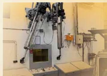
The irradiator **PAGURE** has 6 sources of Cobalt 60 (total activity of 740 TBq), arranged in a room of 25 m<sup>2</sup>. It allows an ageing radiation of small materials, in a range of dose rate from 10 Gy/h to 25 kGy/h.
