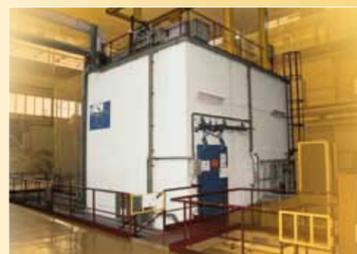
The Van de Graaff accelerator **VULCAIN** delivers electrons from 0.5 to 2.5 MeV. It allows the testing of thin materials such as electrical cables or paint coatings and sealants. Particularly in the framework of 'severe accident' simulations, doses of several dozens of MGy at dose rates of 100 kGy/h and more, can be issued.
