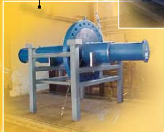
**Irradiation qualification of Ball Valves VIMER** (Modular Isolation Valve with Fast Maintenance), with actuator conducted between 2 pans of POSEIDON sources (VANATOME - TRACTEBEL)
