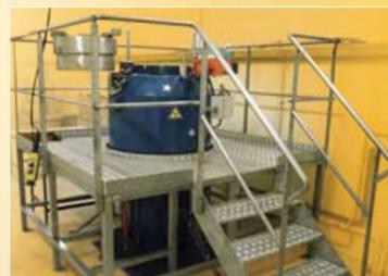
The self-protected **GALAXIE** irradiator equipped with a source of Cobalt 60 (activity less than 0.37 TBq), allows an irradiation at low dose rate (0.36 to 3.6 Gy / h) and electronic components arranged radially in a cylindrical chamber (ht: 420 mm, 160 mm radius).
